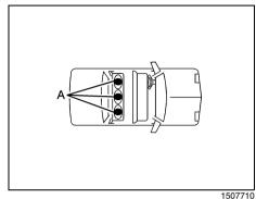
A. Child restraint or occupant using safety belt
